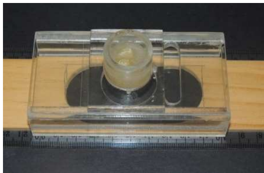
Figure 1. Plexiglas cylinder containing a centrally positioned specimen with the apices facing upward. The cylinder is fixed onto a prefabricated Plexiglas mount to standardize radiographic and photographic documentation. The T-ruler serves to slide the mounting
