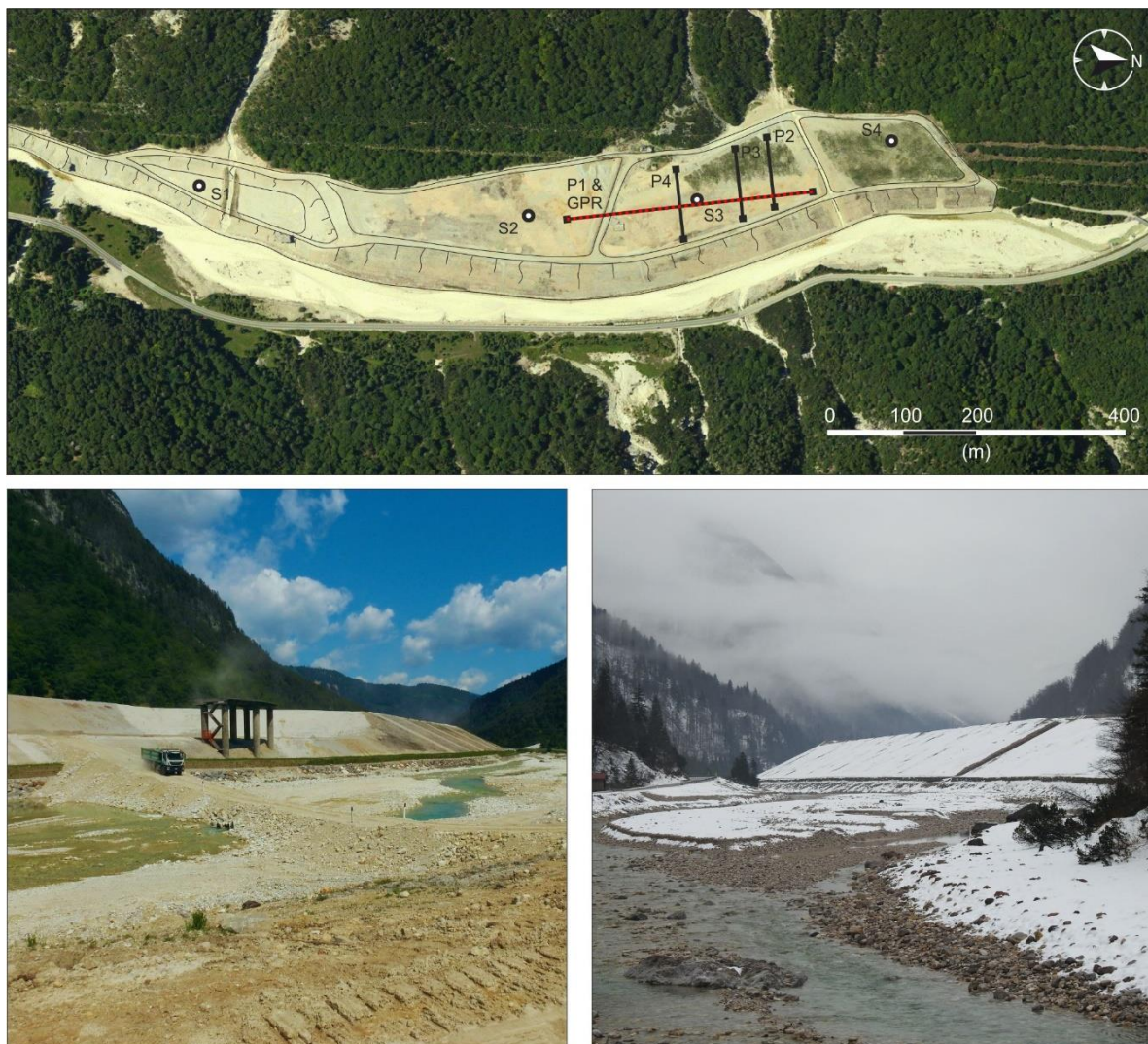
Figure 2. Satellite image showing the extension of the Raibl mine impoundment ( above ). Labels S1-S4 mark the location of the boreholes used in this study, while the solid black and dotted red lines with labels P1–P4 depict the ERT and GPR survey locations respectively. The two pictures below show the impoundment as it appears from the Rio del Lago stream bed, from the south ( left ) and from the north ( right ).
