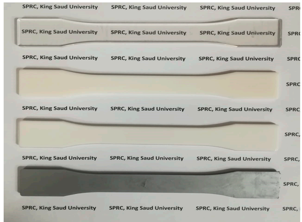
Figure 3. Injection-moulded tensile bar appearance of polymers and composites. From top to bottom: amorphous PET bar is transparent; semi-crystalline PBT bar is white; 60/40 PBT/PET bar is cream tinted; and the Al nano platelet-filled 60/40 PBT/PET bar is silvery.
