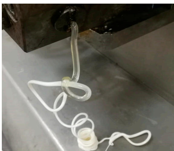
Figure 13. A 60/40 PBT/PET melt emerging from the die is transparent, indicating that the components are either miscible in the melt, or the constituents are in nano domains with similar refractive indices. On cooling, whitening occurs due to crystallisation.
