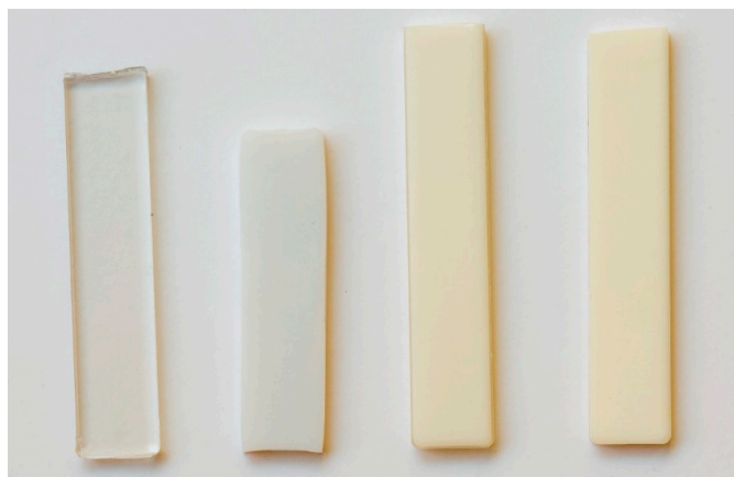
Figure 9. From the left, transparent amorphous PET bar; PET bar after annealing at 150 °C for 30 min. It cold crystallises, turns white, but shrinks and warps; as-moulded 60/40 PBT/PET bar is turbid and has a yellow tint, and shows a transparent amorphous skin; after annealing 60/40 PBT/PET bar at 150 °C for 30 min, the skin cold crystallises, but unlike the amorphous PET, there is no major shrinkage or warpage.
