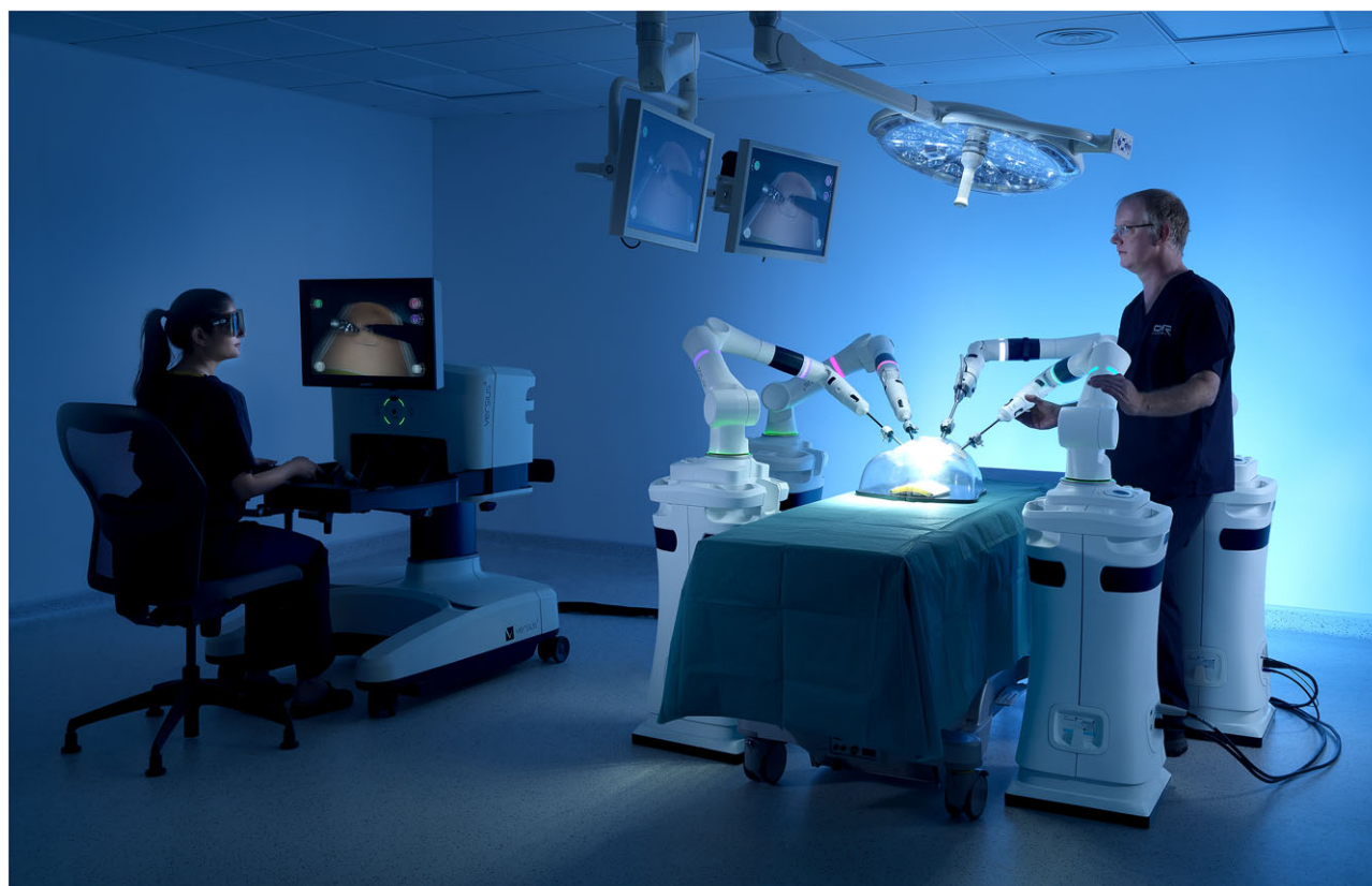
Figure 1: Overview of the Versius Surgical System. Reproduced from Haig et al. [11] A real-world image of the Versius set-up.
