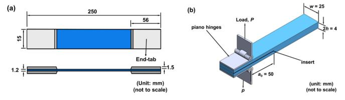
**Figure 3.** Shape and dimensions of the (**a**) bulk specimens for the static and fatigue tests, and (**b**) DCB specimens for the mode I fracture toughness tests.
