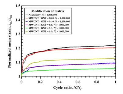
**Figure 10.** Variation normalized mean strain with the applied fatigue cycles for the studied CFEP laminate specimens modified under different nanofiller ratios.
