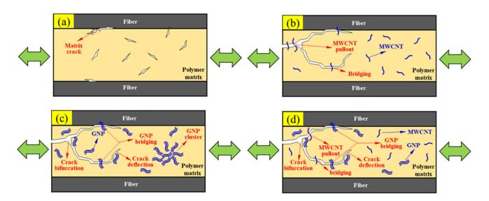
**Figure 15.** Schematic illustration of the fatigue improvement mechanisms for the (**a**) neat CFEP laminate specimen, (**b**) nano-CFEP laminate specimen modified with MWCNTs only, (**c**) nano-CFEP laminate specimen modified with GNPs only, and (**d**) nano-CFEP laminate specimen modified with hybrid nanoparticles.
