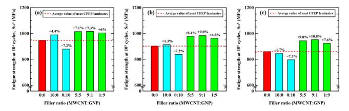
**Figure 8.** Fatigue strengths at (**a**)  $10^4$ , (**b**) $10^5$ , and (**c**)  $10^6$  fatigue-life cycles for the nano-CFEP specimens modified under different nanofiller ratios.
