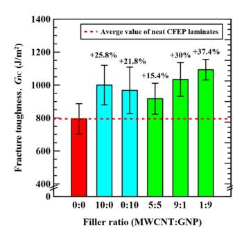
**Figure 11.** Variation of the mode I fracture toughness  $G_{IC}$  of the nano-CFEP specimens with the applied nanofiller ratios in the preparation of specimens.
