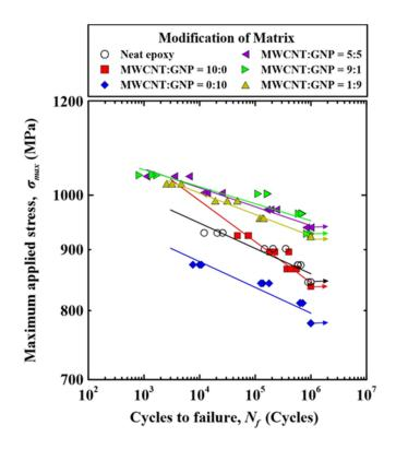
**Figure 6.** Relationships between the loading levels and the fatigue lives for the nano-CFEP laminate specimens with matrices modified under various nanofiller ratios.
