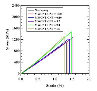
**Figure 4.** Examples of stress–strain curves for the nano-CFEP laminate specimens with matrices modified under various nanofiller ratios.
