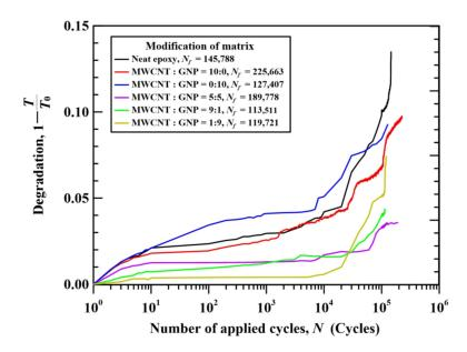
**Figure 9.** Variation of specimen degradation of the studied nano-CFEP laminate specimens with applied cycles.
