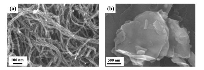
Figure 1. SEM images of the as-received (a) MWCNTs and (b) GNPs.
