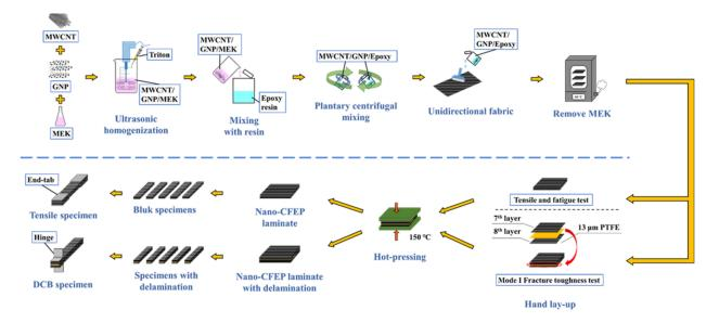
Figure 2. Procedure of specimen preparation.
