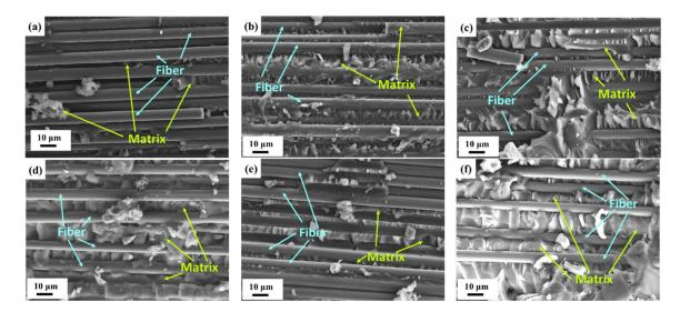
**Figure 12.** SEM images of fracture surfaces for the CFRP laminate specimens with matrices modified under the MWCNT:GNP ratios of (**a**) 0:0; (**b**) 10:0; (**c**) 0:10; (**d**) 5:5; (**e**) 9:1; and (**f**) 1:9.
