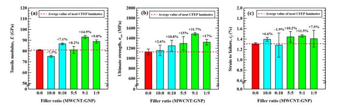
Figure 5. Effect of nanofiller ratio on the (a) tensile modulus, (b) ultimate strength, and (c) strain to failure of the studied nano-CFEP laminate specimens.
