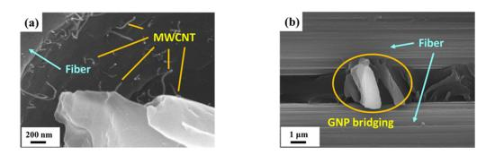
**Figure 14.** (a) MWCNT pullout and bridging observed from the matrix of the nano-CFEP laminate specimen modified under a MWCNT:GNP ratio of 9:1, and (b) GNP bridging observed from the fracture surface of the nano-CFEP laminate specimen modified under a MWCNT:GNP ratio of 0:10.
