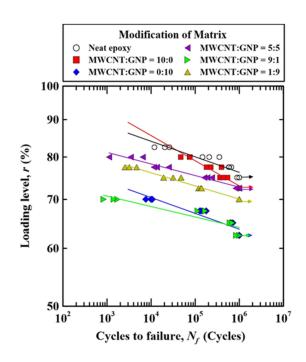
**Figure 7.** Relationship between the loading levels and the fatigue lives for the nano-CFEP laminate specimens with matrices modified under various nanofiller ratios.
