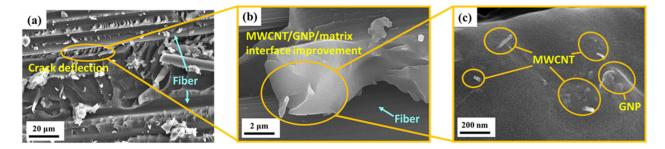
**Figure 13.** (**a**) Crack deflection observed from the fracture surface of the nano-CFEP laminate specimen modified under a MWCNT:GNP ratio of 9:1; (**b**) 3D cluster of MWCNTs and GNPs at the fiber/matrix interface; and (**c**) enlarged image of (**b**).
