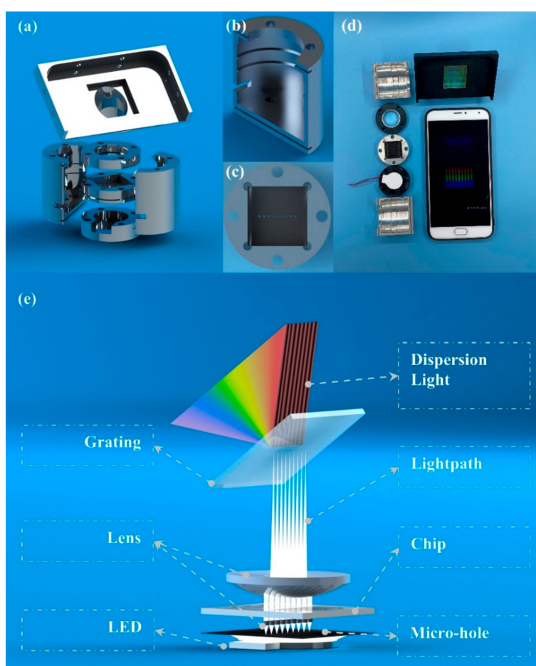
Figure 2. Schematic of attachments of the SBSM (smartphone biosensor system with the multi-testing-unit). (a) The schematic of attachments; (b) The detail of the case; (c) The detail (top view) of the stage of micro-hole array and small-lens array; (d) The picture of attachments and the smartphone; (e) The working principle of the SBSM.
