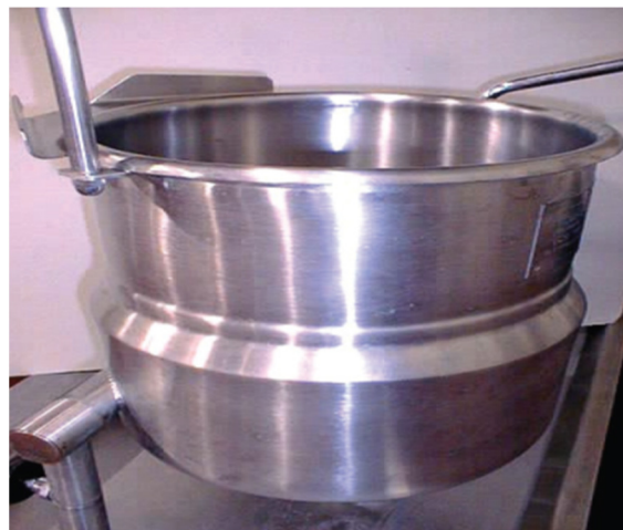
Figure 1. A conventional steam jacketed kettle used to heat batches of food materials. The kettle chamber is typically 1.5 m in diameter with a 1.5 m depth.
