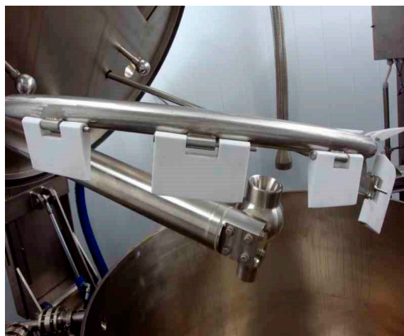
Figure 2. The OAL Steam Infusion Vaction™ pump mounted in a cooking kettle with a scraped surface agitator. Image provided by OAL.
