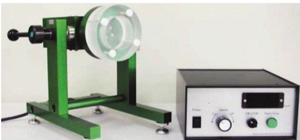
Figure 1. The 2-D clinostats which used to generate SMG conditions on the ground.
