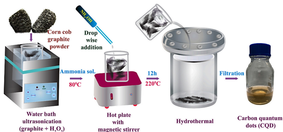
Figure 2. Preparation process of corn cob-derived CQD [52].
