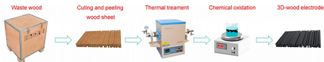
Figure 5. Schematic illustration of 3D-wood electrode synthesis [62].
