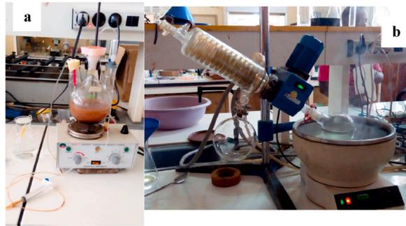
Fig. 1. Lab-scale of the, (a) fermentation; (b) distillation.
