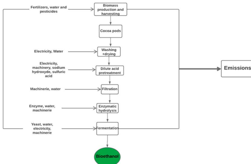
Fig. 2. System boundaries of bioethanol production from cocoa hydrolyzate.
