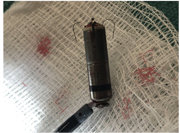
Figure 2 Extracted Micra transcatheter pacing system (Medtronic, Fridley, MN).
