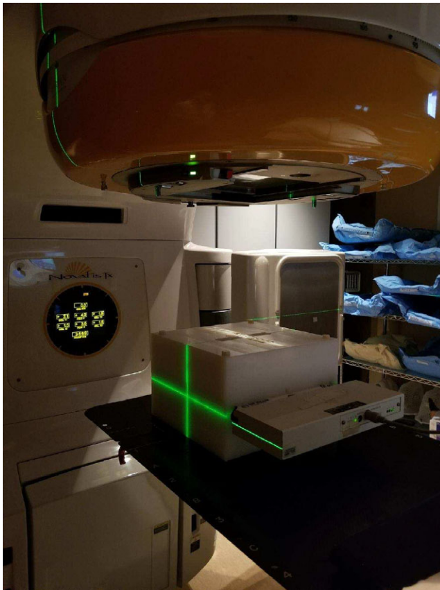
Fig. 3. Experimental QA setup in treatment room showing the MapCHECK QA device inserted in the middle of plastic phantom. [Correction added on 8 th February 2018, after first online publication: Caption was corrected.]
