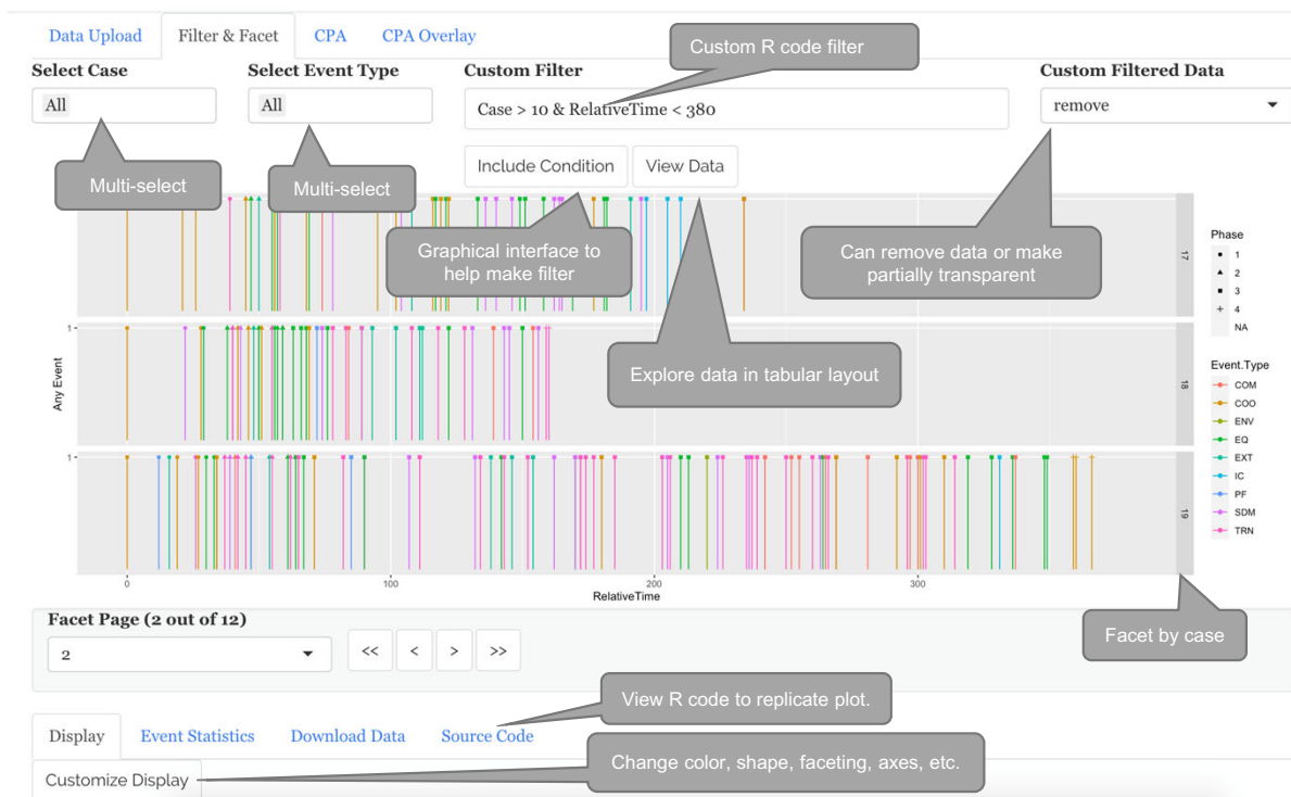
Figure 1. Flow Disruption by Time after Surgery Start, Faceted. The filter and facet tab of read-tv supports faceting (Case), custom filters (Case > 10 and Relative Time < 380), different event colors (Event Type), shape (Phase), source code visualization, and other features shown above. This filtered and faceted data is passed to the CPA tab. The tabs to the right receive data from the tabs to the left.
