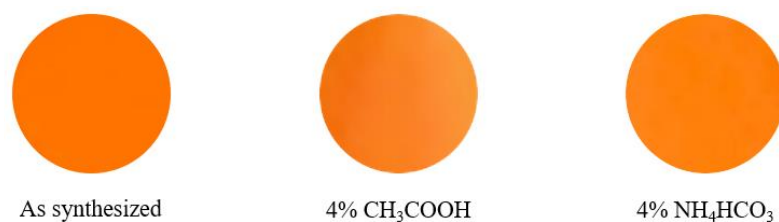
Figure 7. Photographs of the \text{La}_3\text{LiMn}_{0.97}\text{Ti}_{0.03}\text{O}_7 pigment before and after the chemical stability test.
