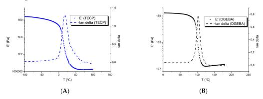
**Figure 5.** E' (**A**-left) and  $\tan \delta$  (**B**-right) of DMA curves for cardanol-based and DGEBA-based materials (blue: TECP; black: DGEBA).
