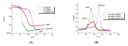
**Figure 4.** E' (**A**-left) and  $\tan \delta$  (**B**-right) of DMA curves for eugenol-based materials (red: DEEP; green: TEEP; magenta: DEEP-Ph).
