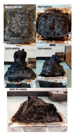
Figure 8. Pictures of residues from cone calorimeter tests.
