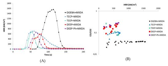
Figure 7. (A-left) Heat release rate versus time. (B-right) CO/CO<sub>2</sub> ratio versus HRR in cone calorimeter tests.
