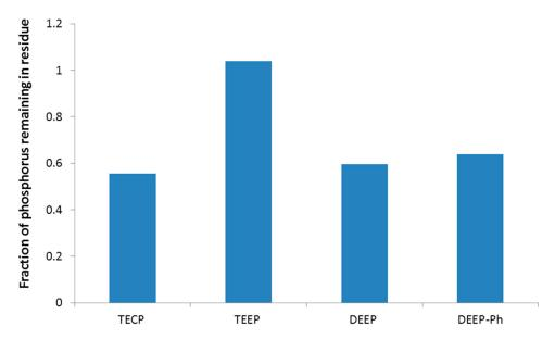
Figure 10. Fraction of phosphorus remaining in residue.
