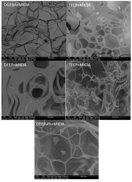
Figure 9. SEM pictures of residues from cone calorimeter.
