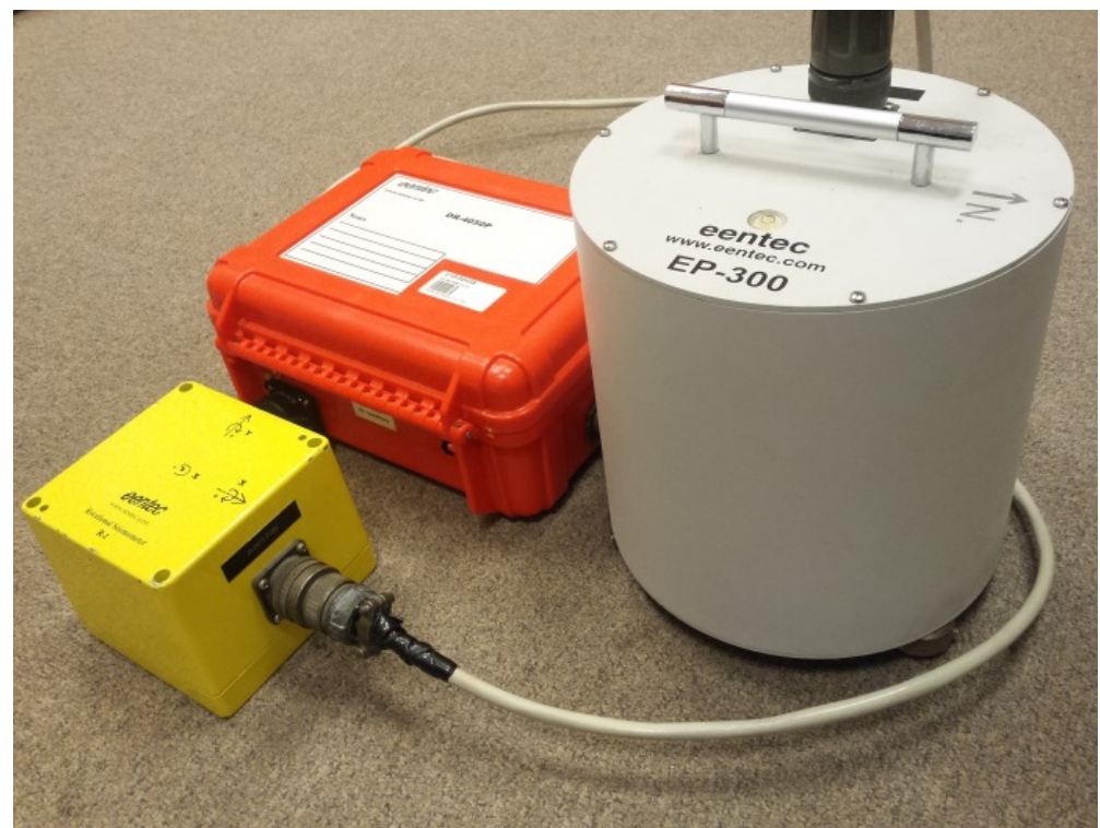
Figure 2. System for 6-DOF measurements installed in the Rudna mining region.
