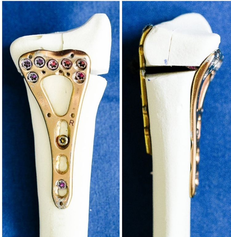
Fig. 3 Exemplified specimens from Group 2 after volar plating using a 2.4 mm Variable Angle LCP Two-Column Volar Distal Radius Plate (DePuy Synthes, Zuchwil, Switzerland) (left), and double plating using a supplemental Variable Angle LCP Dorsal Distal Radius Plate (DePuy Synthes, Zuchwil, Switzerland) (right)
