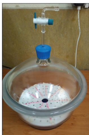
Figure 1: The specimens being kept in a desiccator
