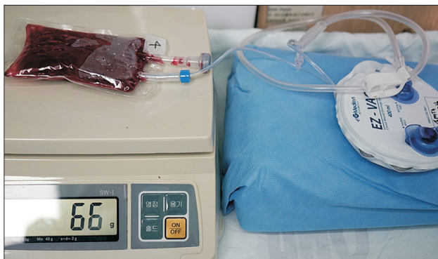
Fig. 1. Photograph of the experimental setup. The blood filled bag was connected to a 120 \pm 30 mmHg vacuum system through a 1.6-mm diameter drain tube and the weight was measured.
