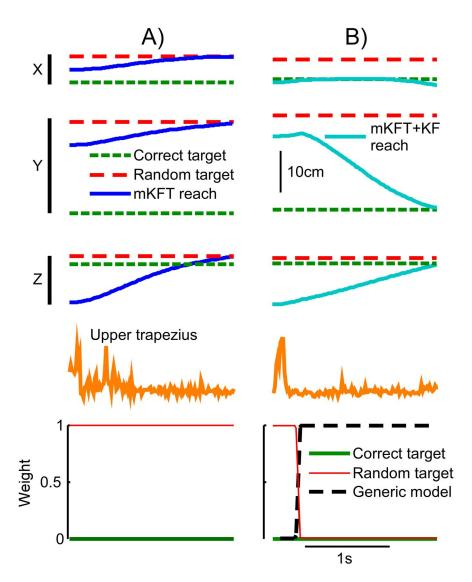
**Figure 6. Example reaches with inaccurate target information, where the random target was assigned a prior probability of 1.** 3dimensional robot endpoint position, RMS feature of EMG windows, and mixture weights with A) mKFT and B) mKFT+KF, incorporating the generic model.
