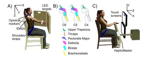
Figure 1. Experimental setups A) Natural reaching data; B) Muscles recorded to simulate levels of SCI; C) Closed-loop experiment. doi:10.1371/journal.pone.0086811.g001
