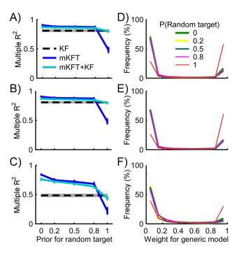
**Figure 4.** Accuracy of the decoding models with varying target uncertainties for A) C6; B) C5; and C) C4 simulated injury levels. d)-f) Corresponding histograms for the weights assigned to the generic model, over the course of all reaches, in the combined mixture case. The histograms are very similar where the prior assigned to the random target is less than 1. Error bars and shading represent standard errors. doi:10.1371/journal.pone.0086811.g004
