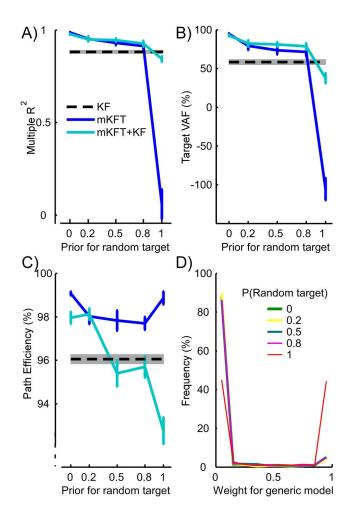
**Figure 5. Closed-loop decoder performance with increasing target uncertainty, at the simulated C4 injury level.** A) trajectory comparison to straight-line reach; B) target accuracy; C) quantification of the trajectory straightness; D) histograms for the weights assigned to the generic model when it was included. The histograms are almost identical where priors for the random target are less than 1. Error bars and shading represent standard errors. doi:10.1371/journal.pone.0086811.g005
