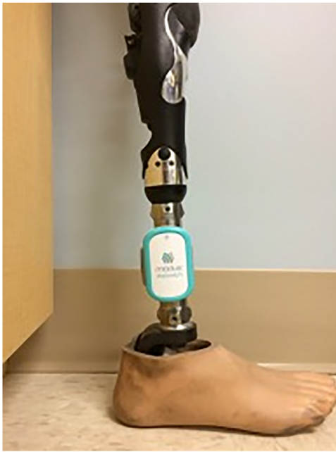
Fig 1 StepWatch activity monitor placed in typical location on prosthesis: lateral ankle region.
