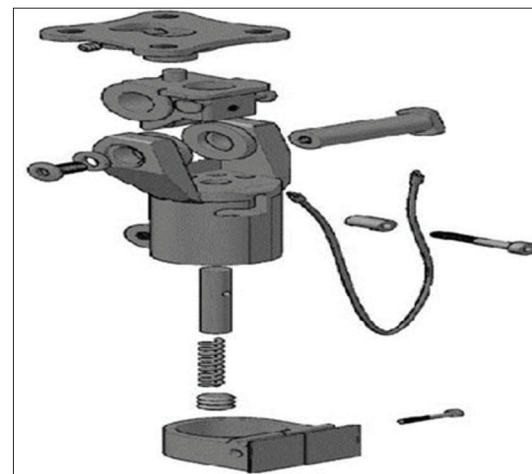
Figure 2: Assembly drawing of safe gait prosthetic knee joint
