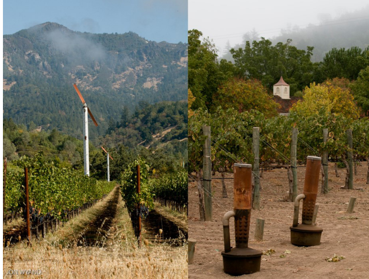
Figure 6. Wind machines and fire drums used by vineyards to increase nighttime temperatures. Wind machines pull warm air from above a field and down towards the crops. Drums, heaters, torches, and containers filled with fuel can create warming by lighting fuel on fire. Photo credit: Jon Wyand.
