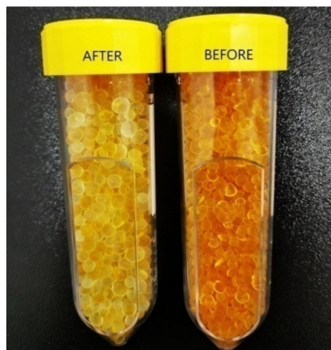
Figure 9. Picture representing the SiO 2 orange pearls after the interaction with a breath sample and before the interaction with a breath sample (color change from orange—before: right to colorless—after: left).
