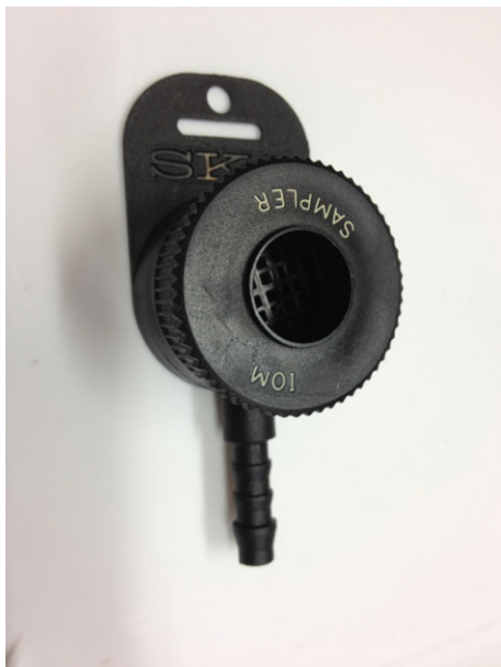
Fig 2. Photograph of Institute of Occupational Medicine (IOM) sampler. [Color figure can be viewed in the online issue, which is available at wileyonlinelibrary.com .]
