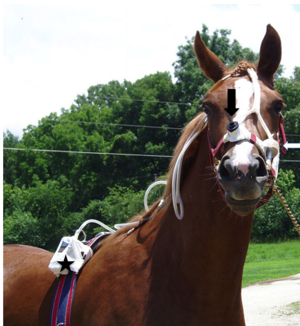
Fig 4. Photograph of horse equipped for air sampling at the breathing zone. Black arrow: IOM sampler c ; White arrow: aluminum cyclone c ; Personal sampling pump (AirCheck 2000 c ). [Color figure can be viewed in the online issue, which is available at wileyonlinelibrary.com .]
