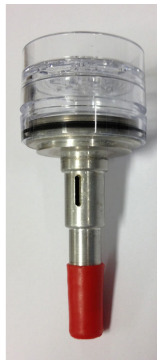
Fig 3. Photograph of aluminum cyclone. [Color figure can be viewed in the online issue, which is available at wileyonlinelibrary.com .]
