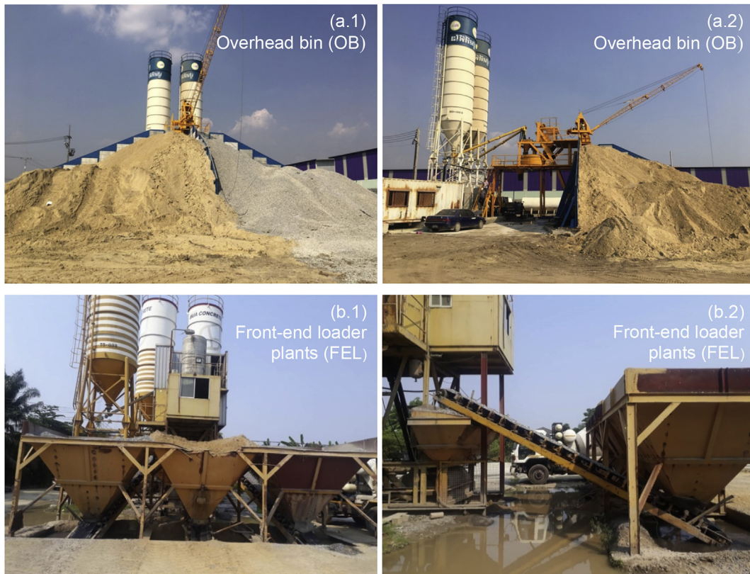
Figure 1. (a) Aggregate unloading to OB plant and (b) aggregate feeding in FEL plant.
