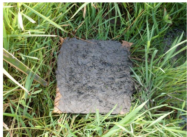
Figure 3 A tracking tile consisting of a bamboo mat (0.3 × 0.3 m) was smeared with mud
