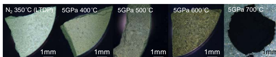
Figure 2. Optical image of LTDP and samples treated at 5 GPa and 400–700 °C.
