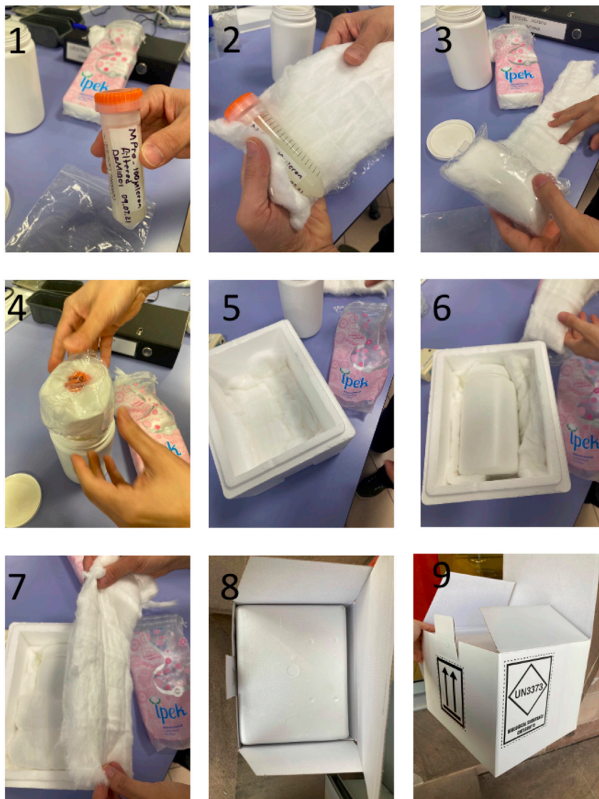
Figure 5. Packaging steps for transport of crystal samples to LCLS
