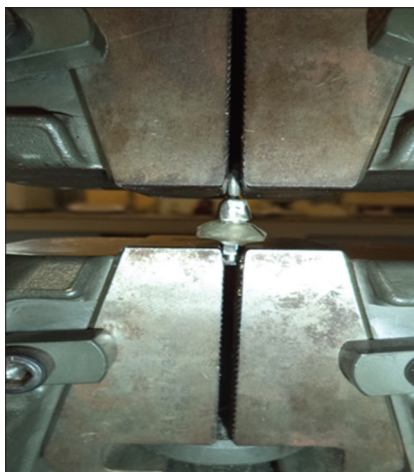
Figure 9: Specimen clamped to the universal testing machine
