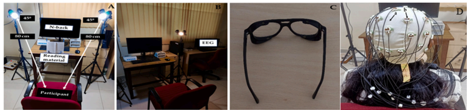
Fig. 2. Light exposure setup with EEG measurements. 2A: White LED (600 lux each) exposure set up along with the distance between the participant’s eye and white light is approximately 80 cm placed at a 45-degree angle. 2B: Amber LED (470 lux each) exposure setup required for washout of white light. 2C: Customizable wrap-around blue-blocking lens (BBL). 2D: Electroencephalography (EEG) Electrocap on the participant’s scalp with 32 electrodes, (a) EEG scalp cap; (b) EEG electrodes.
