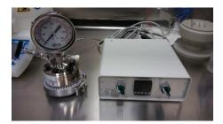
Figure 1. Hydrothermal growth set up with the stainless steel autoclave and temperature regulator.
