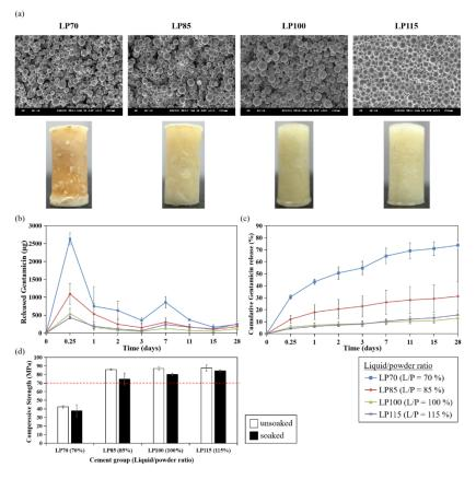
**Figure 4.** Effects of liquid/powder ratio on antibiotics elution and compressive strength of PMMA bone cement. (a) SEM images and morphology of PMMA cement. (b) Gentamicin elution profile. (c) Cumulative gentamicin release percentage. (d) Compressive strength. White bar: unsoaked cement; black bar: PBS-soaked cement. The dashed line indicates the ISO standard for compressive strength (70 MPa).
