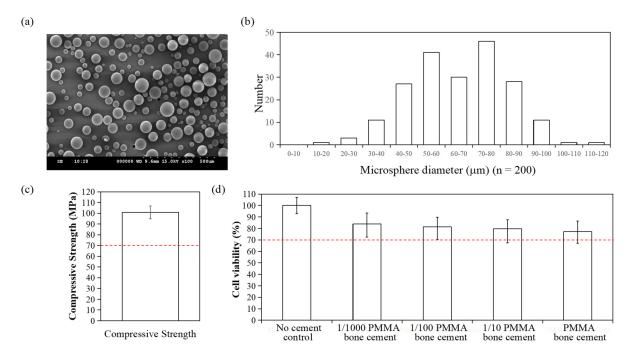
**Figure 2.** Characterization of PMMA bone cement. (**a**) SEM image of PMMA bone cement. (**b**) Particle diameter distribution of PMMA. (**c**) Compressive strength of PMMA bone cement. (**d**) Cell viability of L929 cells measured by MTT assay for evaluating the biocompatibility of PMMA bone cement. The dashed lines indicate the ISO standard for compressive strength (70 MPa) and cell viability (70%).
