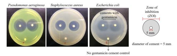
**Figure 1.** Representative photos of agar disk diffusion bioassay. ZOI of *Pseudomonas aeruginosa, Staphylococcus aureus* and *Escherichia coli* was measured as indicated in the illustration. The diameter of the bone cement disc was 5 mm.
