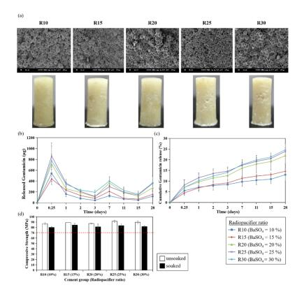
**Figure 5.** Effects of radiopacifier ratio on antibiotics elution and compressive strength of PMMA bone cement. (**a**) SEM images and morphology of PMMA cement. (**b**) Gentamicin elution profile. (**c**) Cumulative gentamicin release percentage. (**d**) Compressive strength. White bar: unsoaked cement; black bar: PBS-soaked cement. The dashed line indicates the ISO standard for compressive strength (70 MPa).
