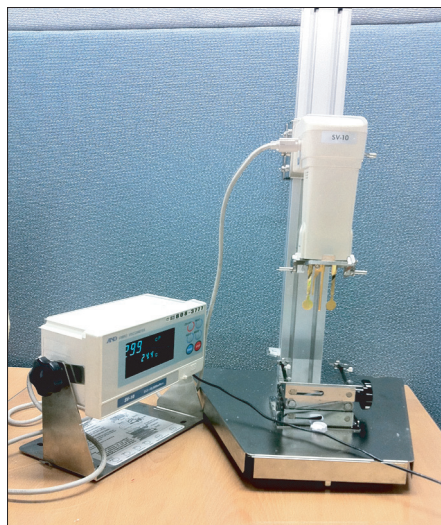
Fig. 2. The viscosity of each bolus was measured with a viscometer SV-10/100 ® (A&D Co., Tokyo, Japan).
