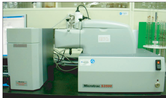
Fig. 3. Laser diffraction S3500 ® (Microtrac Inc., Largo, USA) was used to analyze distributions of particle size in the food boluses.
