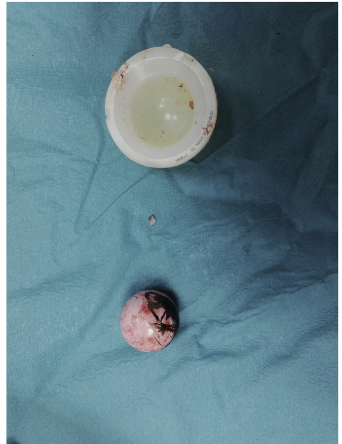
Figure 2. Retrieved polyethylene insert and head showing fractured tabs and deformed shape.
