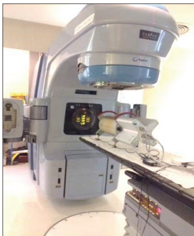
Figure 1: The Delta 4 phantom was placed in a certain location on the linear accelerator treatment couch
