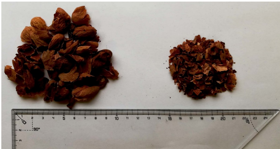
Figure 3. Aggregates used. (On the left) almond residue in its true state used for AS0_GA, (on the right) almond residue in ground state used for AS1_PVA.
