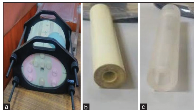
Figure 1: Photograph of CIRS intensity-modulated radiation therapy thorax phantom and the removable dosimetry insert: (a) CIRS intensity-modulated radiation therapy thorax phantom, (b) insert for air ionization chamber available from CIRS, and (c) fabricated insert for liquid ionization chamber
