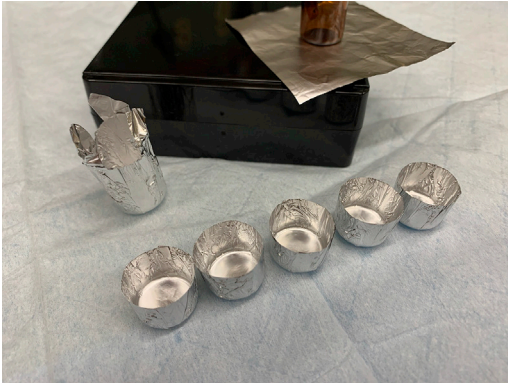
Figure 1. Homemade brain tissue freezing foil molds that are optimized for rapid freezing for downstream sagittal cryosections (image courtesy of Patrick Burrola)
