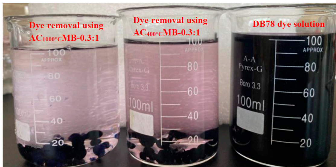
Figure 13. DB78 dye solution and dye removal using AC 1000°C MB-0.3:1 and AC 400°C MB-0.3:1.
