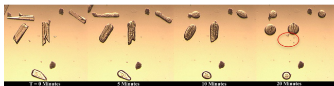
Figure 4. Four frames at t = 0, 5, 10 and 20 min of the dissolution of DMOF-1-NHCH 2 OCH 3 crystals in the presence of a solution of toluene and pyrazole. Small crystals of 5 can be seen starting to form near the centre of the final frame.
