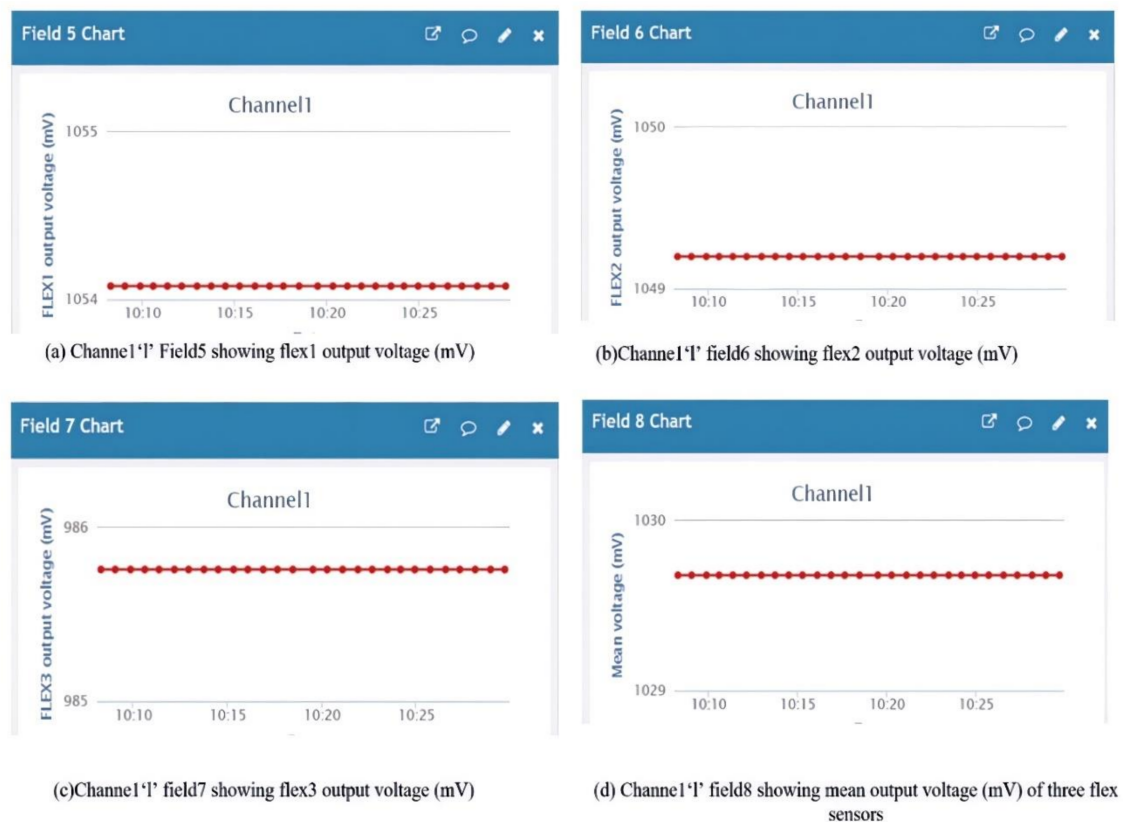
Figure 19. Channel '1' showing the voltage output (mV) of all three flex sensors with mean level.
