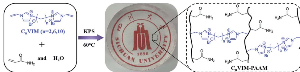
Fig. 1 Schematic diagram of C_n VIM-PAAM hydrogel preparation and image of the resultant hydrogel.
