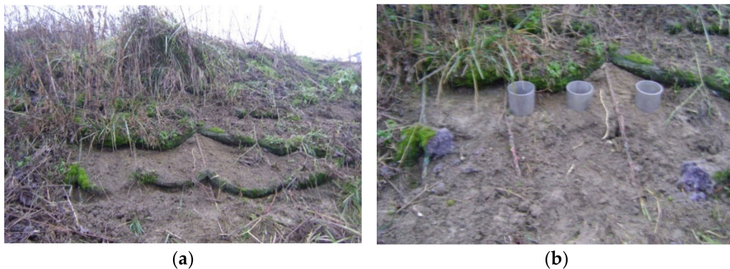
Figure 5. Sampling on 18 January 2020 at location 4. (a) The lower rope with three sections (left section, LS; center section, CS; right section, RS). (b) The sample cylinders and the cut-off rope for the rope tension strength determination and scanning electron microscopy (SEM).
