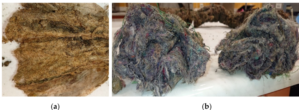
Figure 11. View of the ropes 47 months after installation. (a) Wool rope; (b) recycled natural and synthetic fiber (RNSF) ropes (left: From location 4; right: From location 5).
