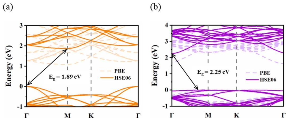
Fig. 2 (a) Band structure schematic diagram of monolayer  $\text{ZrS}_2$ , (b) band structure schematic diagram of monolayer  $\text{InSe}$ ; in both (a) and (b), the dashed lines represent the calculated result by the PBE method, and the solid lines represent the results from the HSE06 method.
