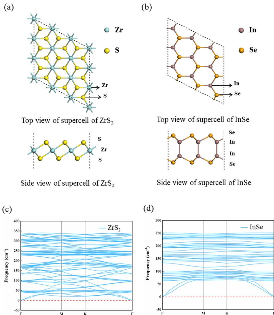
Fig. 1 (a) Lattice structural model diagram of monolayer ZrS<sub>2</sub>, (b) lattice structural model diagram of monolayer InSe. Specifically, Zr, S, In, and Se atoms are plotted by blue, yellow, brown, and orange balls, respectively. (c) The phonon dispersion of monolayer ZrS<sub>2</sub>. (d) The phonon dispersion of monolayer InSe.
