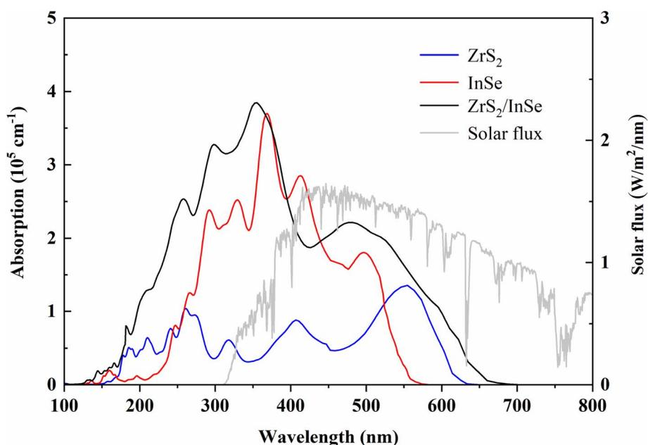
Fig. 8 The optical absorption coefficients of monolayer ZrS<sub>2</sub>, monolayer InSe, and ZrS<sub>2</sub>/InSe heterostructures, calculated by the HSE06 method.
