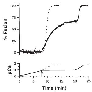
FIGURE 2. Interrupted ramp. Interrupting a calcium ramp (*arrow*) and maintaining this calcium concentration (*solid line*) results in submaximal extents of fusion that are indistinguishable from those produced by step changes to the same calcium concentration. See Fig. 8 A.
