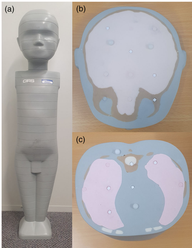
FIGURE 1 (a) The anthropomorphic phantom used for direct organ dose measurements. (b) The placement of TLDs within the phantom (skull). (c) The placement of TLDs with the phantom (thorax). TLDs, thermoluminescent dosimeters
