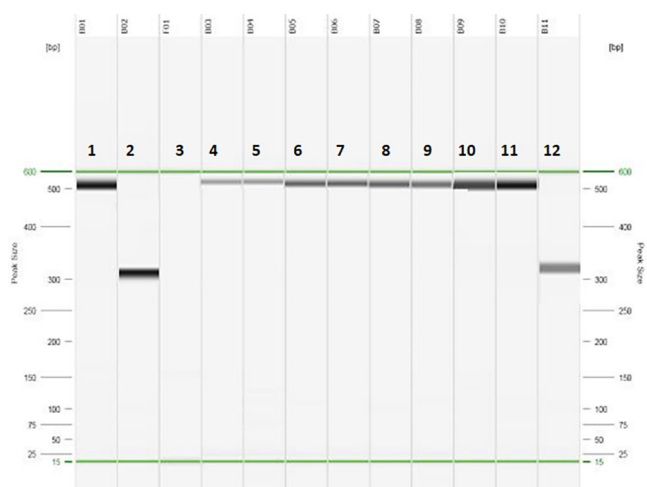
FIGURE 3 Electrophoresis of the polymerase chain reaction products using the QIAxcel machine. Lane 1 is a control-negative Escherichia coli isolate. Lane 2 is a control-positive Aspergillus niger ATCC 1015 with a band size of 301 bp. Lane 3 is a control-positive Rhizopus oryzae HUMC 02 with a band size of 552 bp, while Lane 2 is a control-positive Aspergillus niger ATCC 1015 with a band size of 301 bp. Lane 3 is a control-negative Escherichia coli isolate. Lanes 4–11 are positive isolates for R. oryzae . Lane 12 is an appositive isolate for A. niger
