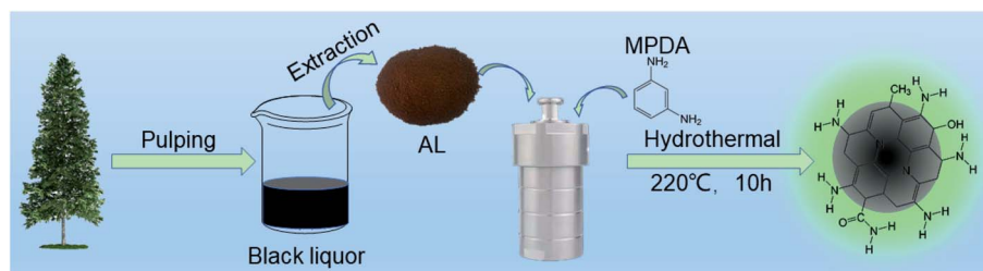
Scheme 1 Preparation process of NCQDs from alkaline lignin.
