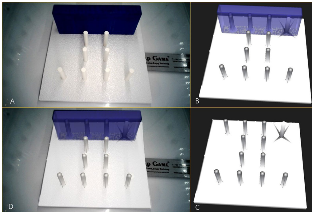
Fig. 2 A The laparoscopic visual field of the simulator. B The 3D model of the rigid model with a covering. C The 3D model of the rigid model without a covering, showing the structures inside. D The fusion image of 3D model and laparoscopic visual field, showing the covered structures
