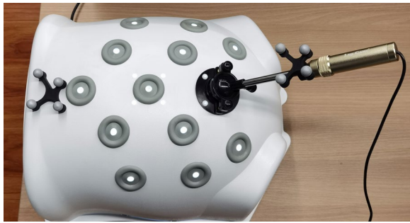
Fig. 1 Laparoscopic simulator with rigid or phantom models fixed inside and optical markers fixed on the outer case and the laparoscopy
